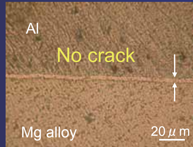
Intermetallic layer formed between Al and Mg alloy
