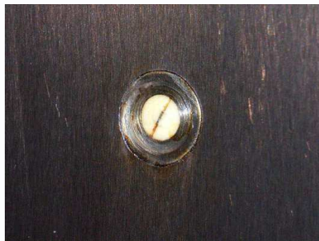
図10 接点むき出し式熱電対
