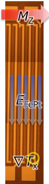
Thermopiles with 5 $\mu$ m-width FePt and Cr wires
