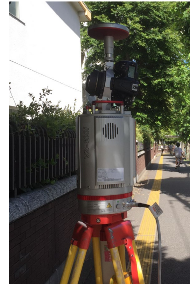
TLS (Terrestrial Laser Scanner)
